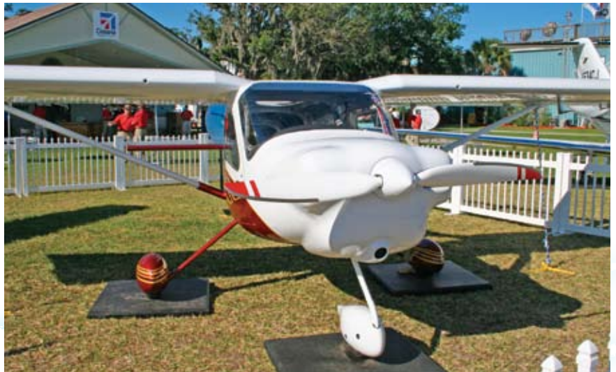
Cessna Aircraft's proof-of-concept Cessna Sport was transported to Sun 'n Fun with a new Continental O-200 engine on the nose. Flight testing was scheduled to begin after the fly-in.
