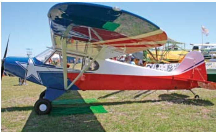
The Texas Sport is available as an amateur-built kit from the Texas Sport Aircraft Company, a sister company to American Legend Aircraft. It can be built with a 1,600 or 1,320 gross weight; at the lower weight, it's sport pilot eligible. www.TxSport.aero .
